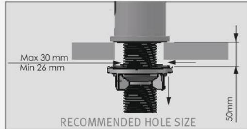
If your dispenser is supplied with anti-rotation solution, drill an additional hole for anti-rotation pin.
