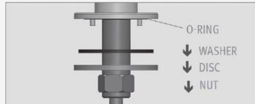
Drill a hole in the counter for the mixing handle. Remove the nut, disk and seal.
